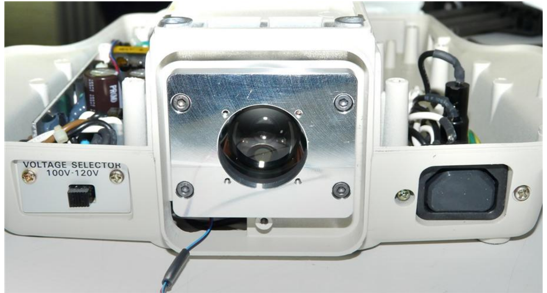
(3) Attach the Adapter Plate using the four M3 x 12mm screws and the 2.5mm hex key. Then install the AC blocking plug in the obsolete AC power receptacle
