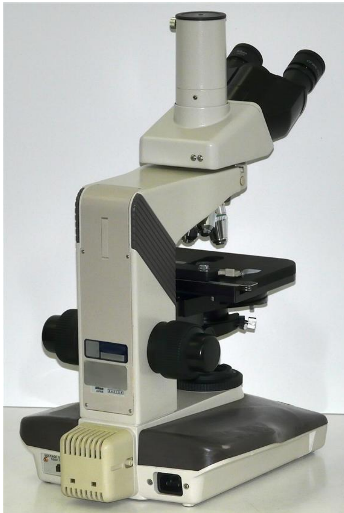
(1) Labophot-2 with original lamp housing. Be sure the AC power cord is disconnected before starting.
