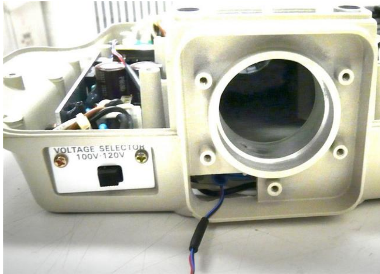
(1) Route the pot cable as shown. Only enough to connect to the illuminator needs to extend out of the microscope.
