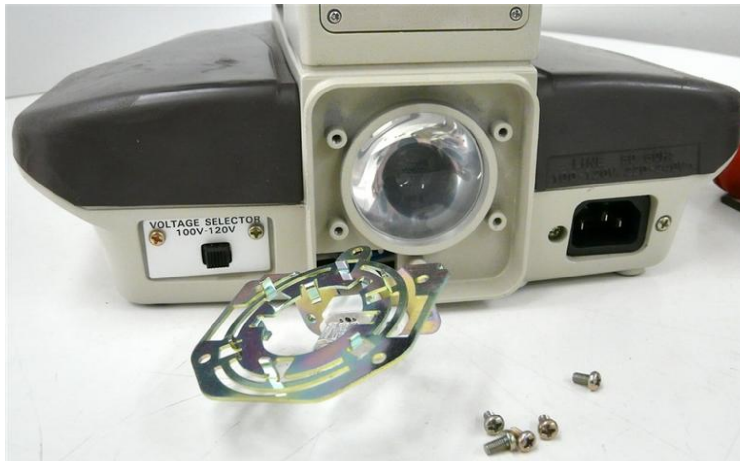
(3) Remove OEM lamp assembly by removing the 5 screws. Warning - the lens is held in place by this assembly.
